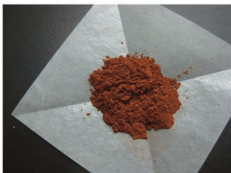
Fig. 4. Powder of heat-treated sludge obtained by heat-treating the dried sludge (Fig. 3) at 450°C for 24 hours.
